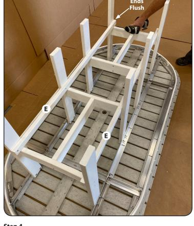
Place the two cross supports (E) on top of the H Stetchers, one on each side, and up against the legs, as shown. Fasten the cross supports to the end legs first, keeping them flush, using two 2" screws for each of the 4 end legs., then fasten the remaining 4 middle legs with the remaining 8 screws, 2 per leg.
