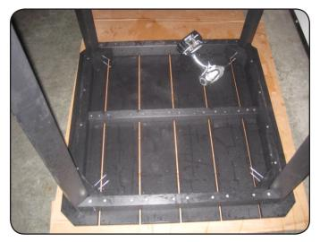
Lay table (A) upside down on a soft surface and fit legs (C) in pockets provided where shown and fasten from inside with (8) 3" screws.
