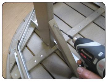
**Step 4**Fasten brace to inside of leg where shown with a 2" screw and a 1 1/4" screw from inside through hole in angle iron into other end of brace. Repeat other 3 sides.
