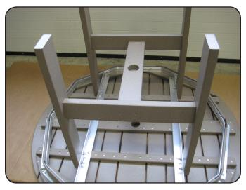
**Step 3**Now position the assembly where shown in between legs and fasten with (8) 2 1/2" screws through predrilled holes measuring 11" from the bottom of leg to assembly.
