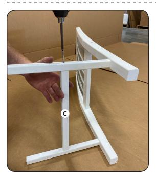
Step 2 Now fasten the cross support (C) in between the two side rails, through the holes provided with (2) 2" screws, one on each end.
