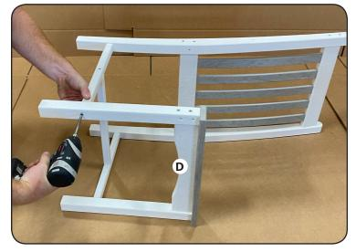
**Step 3**Next fasten the front assembly (D) to both of the side rails using (2) 2 1/2" screws, through the holes provided, one per leg.
