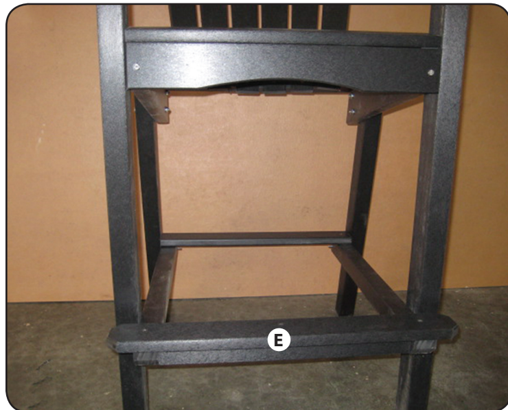
Step 4 Fasten footrest (E) to legs with (4) 1/4"x3-1/2" bolts and nuts.
