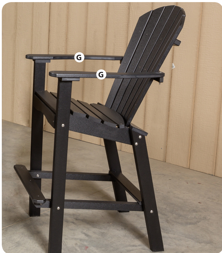
Step 5 Fasten the back of one of the armrests (G) to the backrest with (1) 1/4"x2-1/2" bolt and (1) 1/4" flange nut. To fasten the front leg to the armrest, first divide space evenly on each side then fasten with (3) 1-1/4" screws from bottom up through pre-drilled holes. Repeat with other armrest. Your chair is now complete.
