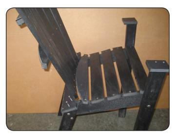
**Step 3** Fasten back (B) in position shown with (6) 2" screws.
