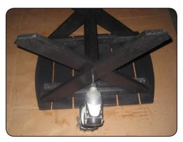
**Step 3**Feed a 3" screw through holes in center of legs and fasten leg support (C). Repeat other side.
