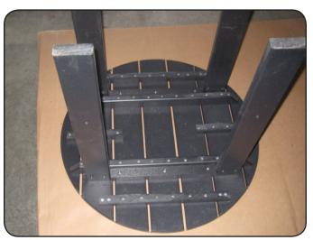
**Step 1**Lay table (A) upside down on a soft surface and attach legs (B) in positions shown with (3) 1 3/4" screws.
