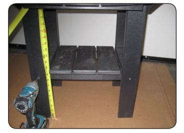
**Step 2**Attach shelf (C) where shown (shelf needs to be flush with outside of legs). Measuring 9 3/4" to top of shelf fasten with (4) 1 3/4" screws (predrilled holes provided).
