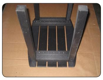
**Step 1**Lay Table (A) upside down on a soft surface and attach 4 legs (B) in positions shown with (8) 2 1/2" screws. Notice left & right.
