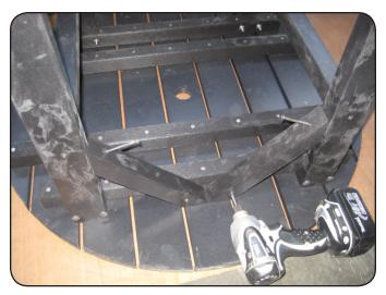
**Step 3**Fasten 2 braces (C) where shown using (4) 2 1/2" screws. notice they are drilled with counter sink holes for left & right. Repeat other side.
