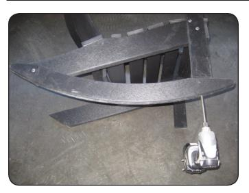
**Step 3**Lay the assembly on side as shown and fasten rocker (C) in back with 2 1/2" bolt & nut on outside of seat support. Fasten the front with (2) 4" screws to the bottom of leg. Repeat other side.
