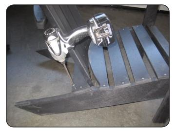
**Step 2**Fasten Back (B) onto seat (A) where shown with (4) 2 1/2" screws. Leave 3/4" gap between last slat in seat and back boards.
