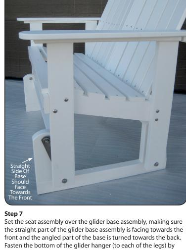
sliding (1) 3/8" washer onto (1) 3/8" x 2 1/4" machine bolt. Push the bolt through hole from the inside to the outside. Now, add another 3/8" washer, then fasten (1) 3/8" lock nut tightly on to the bolt.
