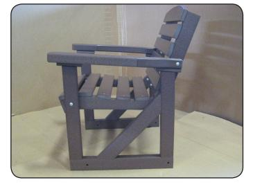
**Step 2**Fasten the leg (C) in position shown using (1) 4" carriage bolt in back of arm, and (1) 3 1/2" carriage bolt in front leg, and (2) 1/4" flange nuts. Repeat other side.
