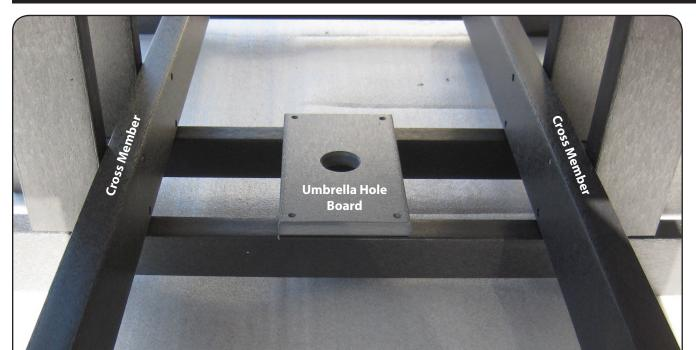
Step 4 Set the table up on its legs. Lay the umbrella hole board (E)on top of the two middle leg sets, as pictured left. Measure it carefully to align it with the umbrella hole that is in the table top above. Fasten with (4) 2" screws.
