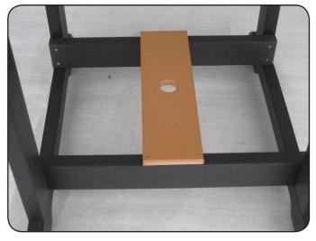
**Step 4**Now set table on legs and fasten bottom board with umbrella hole on the cross members. Measure carefully to align with top umbrella hole. Fasten with (4) 2" screws.
