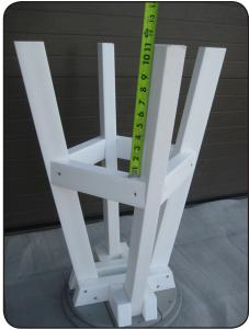
**Step 2**Now fasten braces as shown with (8) 2" screws. NOTE: measuring 11 1/4" as shown.
