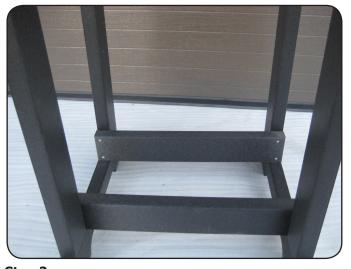
Fasten cross members (B) where shown on inside of leg with (8) 2 1/2" screws.
