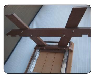
**Step 1**Lay top (A) upside down on a soft surface and attach legs (B) with (8) 5/16" x 3 1/2" carriage bolts and (8) 5/16" flange nuts.
