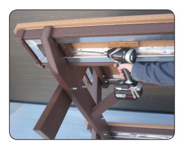
**Step 3** Place seats (D) in notch and fasten with (8) 2 1/2" screws.
