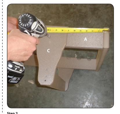
Position the back leg assembly (C) against the seat assembly keeping it flush with the top as shown and 7" in from the back end of the seat assembly and fasten with (6) 1 1/4" screws, 3 on each side.
