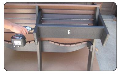
**Step 5**Between the middle leg and the outside leg, place one of the leg supports (E) into the groove and fasten with (4) 2" screws. NOTE: The screws in the middle need to be screwed in from the underside as shown in the picture on the right. Repeat with the other leg support.
