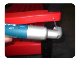
**Step 4**Fasten back of arm rest with (1) 2 1/2" screw. Repeat on other side.
