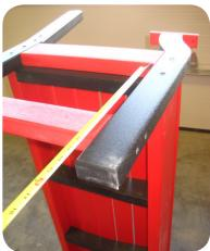
**Step 1**Set seat (D) on end, place side assembly (A) on top, measure 1" as shown. Space evenly on sides and fasten through holes provided with (4) 4" screws.
