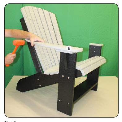
**Step 4**Place an armrest (E) onto the armrest block with the widest portion of the armrest facing towards the front, and turning it so the indent is facing the inside of the chair. On the back of the armrest tap (1) 1/4"x2-3/4" bolt through the pre-drilled hole on the backrest, add (1) 1/4" flange nut. Repeat on the other side.
