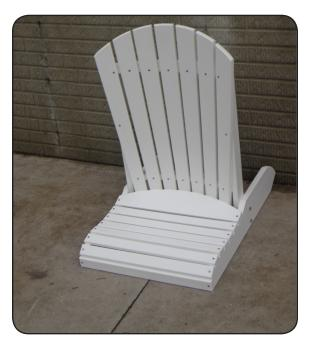
**Step 1**Using (4) 1/4" x 2 1/4" bolts and (4) 1/4" nuts, attach back (A) to seat (B).
