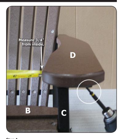
**Step 4**Measure 3/4" from inside as shown. Using (2) 1 1/4" screws attach arm rest (D) to chair leg (C). Repeat on other side.
