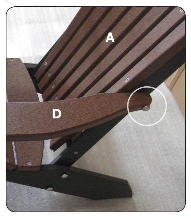
**Step 3**Using (1) 1/4" x 2 1/2" bolts, and (1) 1/4" nuts, attach arm rest (D) to chair back (A). Repeat on other side.
