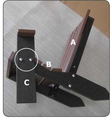
**Step 2** Using (2) 1/4" x 2" bolts and (2) 1/4" nuts, attach leg (C) to seat (B). Repeat on other side.
