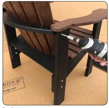
**Step 5** Place a 1/4" washer onto a 1/4" x 3" lag bolt and fasten the backrest to the arm assembly through the hole provided, repeat with the other arm assembly.
