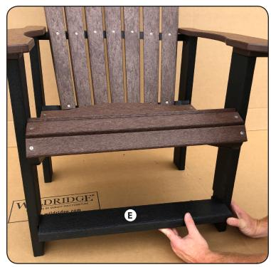
**Step 6**Slide the stretcher (E) into the slots on the inside of the front legs. Fasten from the outside, through the holes provided with (4) 2" screws, two per leg.
