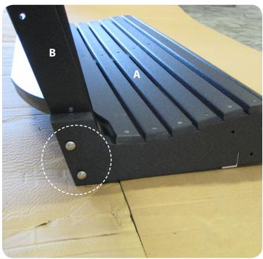
Attach the seat (A) to the backrest (B) using (2) 5/16" x 3 1/2" bolts and (2) 5/16" flange nuts. Repeat step on opposite side.
