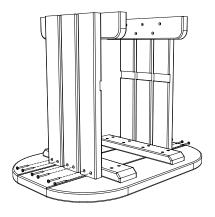
2. Insert (B) Shelf in Notches on Sides Attach with 6 - 1-1/2" Screws Per Side in Pocket Holes.
