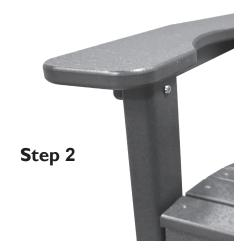
2. Attach the arms to the front legs using two 2 3/4" bolts and flanged lock nuts. The arm support under each arm should be on the outside of the front leg. The bolt should go through the front leg first and then through the arm support underneath the arm. HAND TIGHTEN the flanged locks nuts for now.
