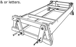
4. Attach (F) Armrests to Glider Base using (2-Washers)&(2-Nuts) per side, be sure to match all numbers & or letters. "Assembly order is Armrest Assembly-Washer-Nut"
