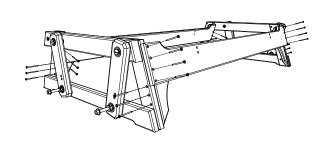
2.Attach (H) Crosspiece Supports to Front-Back Crosspieces using 4 - 2" Screws per side, be sure to match all numbers & or letters.
