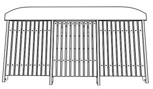
6. Attach Back Assembly to (A) Seat Assembly using 6 - 2" Wafer Bolts, be sure to Match all numbers & or letters, tighten Wafer Bolts with included Hex Key.
