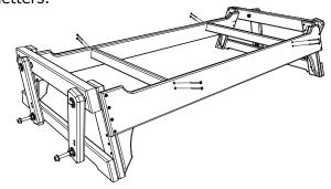
3. Attach (D) Bearing Arm Supports to Glider Base using 4 - 2 1/2" Screws per side, be sure to match all numbers
