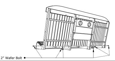
7. Attach Back-Seat Assembly to Armrests using
