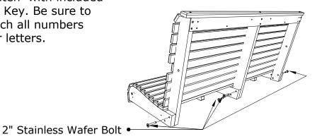
2. Assemble (C) Armrest Assemblies using 1 - 3 1/2" Wafer Bolt, 1 - 2 1/2" Wafer Bolt 1 - 2" Wafer Bolt per side,
