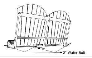
7. Attach Back-Seat Assembly to Armrests using
