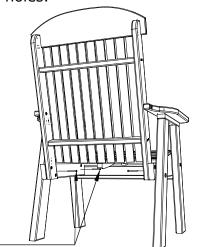
2 1/2" Stainless Wafer Bolt 2" Stainless Wafer Bolt
