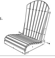
6. Slide Seat & Back Assembly between Armrest's & install 1 - 3 1/2" Wafer Bolt 1 - 2 1/2" Wafer Bolt & 1 - 2" Wafer Bolt per side, Be sure to match all numbers & or letters, Tighten Wafer Bolts with included Hex Key.
