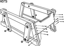
2. Attach (E) Back Cross Pc. to Glider Base Sides using 7 - 2" Screws per side, Be sure to match all numbers & letters.
