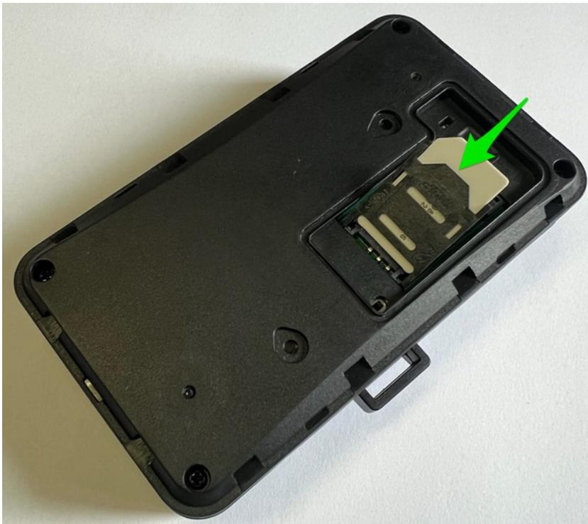
Slide the SIM card retainer at the back of the GPS Tracker backward and rotate it up. Insert the SIM card into it and then rotate it down and slide it forward. See the blue arrows in next image.
