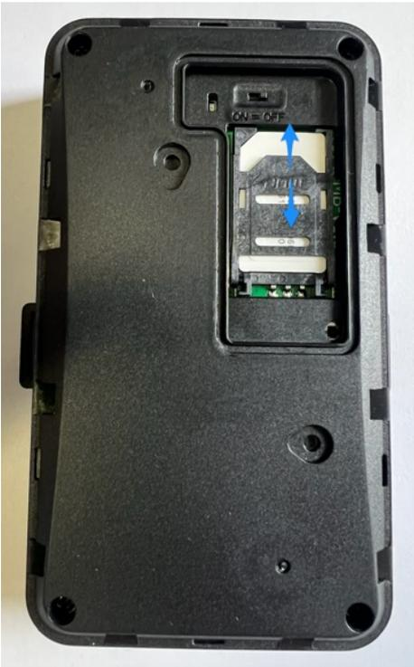
Toggle the battery switch above the SIM card slot to ON position. This is only for initial use.
