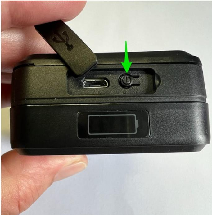
You can charge the battery of the GPS Tracker with the power slot next to the On/Off button.
