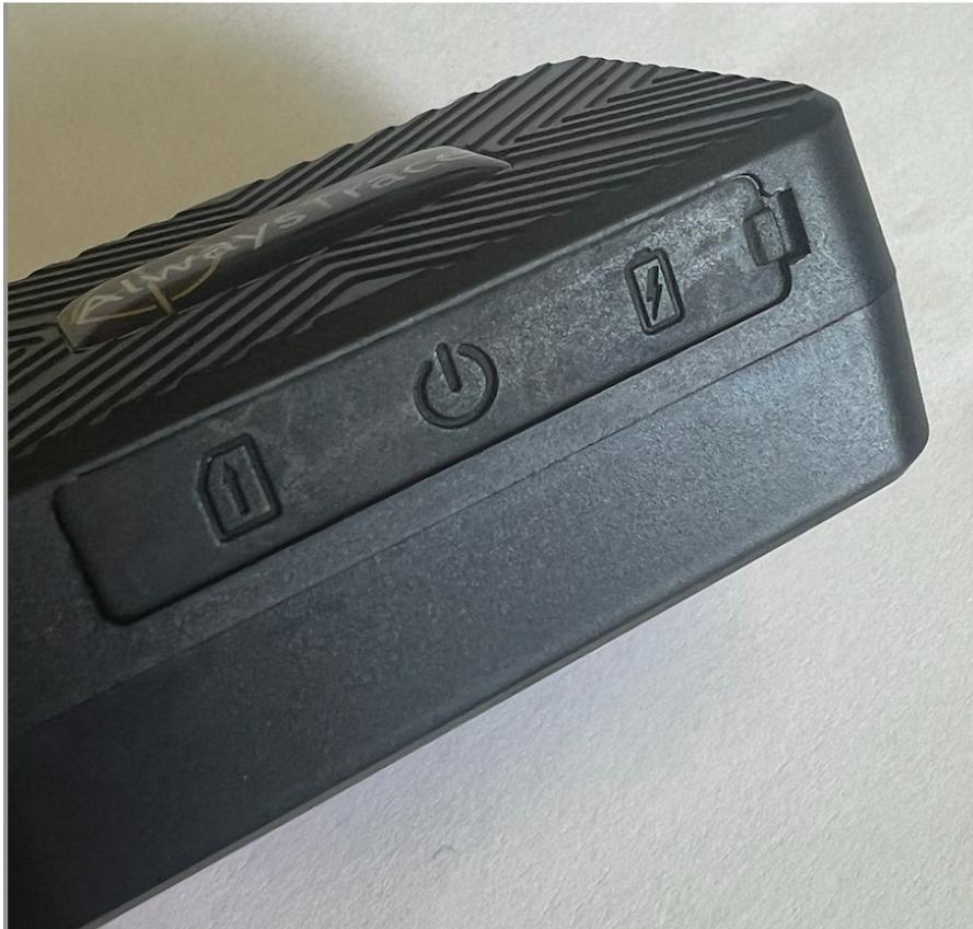
Open the silicone plug and insert the SIM card.
