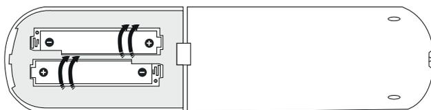
The type of batteries used in the remote control is AAA/R03/1.5V.
