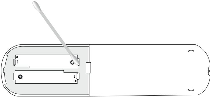
If the remote control no longer works after all operations (cleaning the remote control contacts and batteries replacement of the remote control), contact the service center of the manufacturer or dealer in your area.
