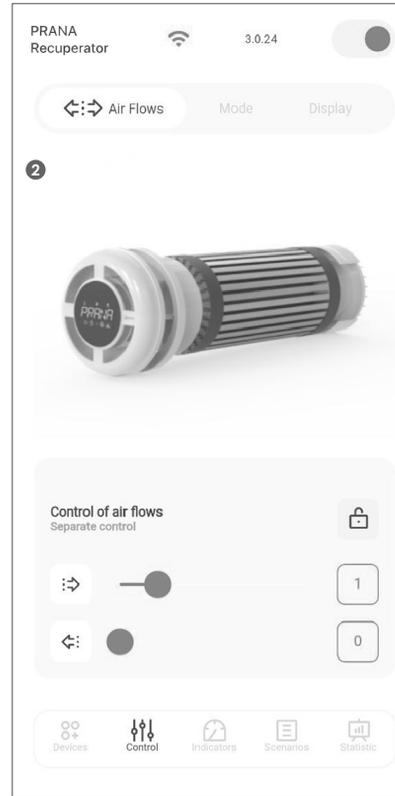
The tab allows you to control airflow in manual and separate control modes.
