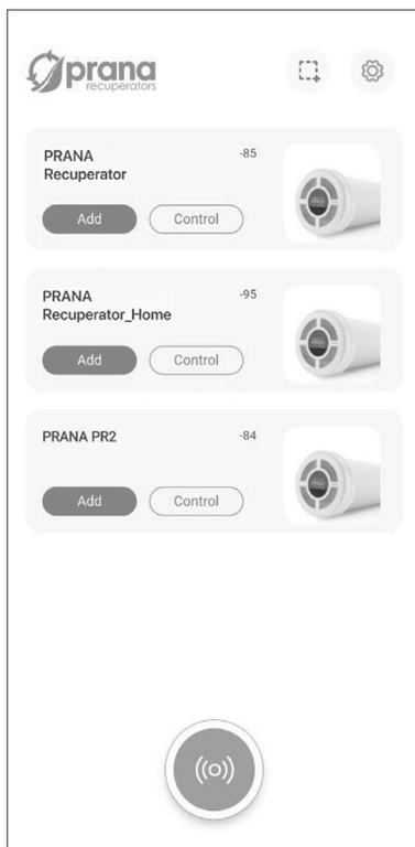
Select the Bluetooth connection method (for the initial connection), and click the «Scan» button
