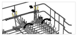
At the back of the right side of the lower basket, the plate supports can be pushed together to provide more space for, say, stoneware or a large pan.
