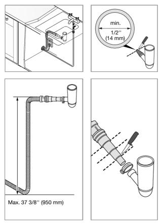
The drain hose can also be connected to a connection nipple on the sink unit's water trap. The connection nipple must have an internal diameter of at least 1/2'' (14 mm).
