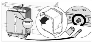
Adjust the front feet by turning them clockwise to raise and counterclockwise to lower the dishwasher.
