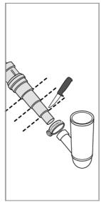
The drain hose can also be connected to a connection nipple on the sink unit's water trap. The connection nipple must have an internal diameter of at least 1/2" (14 mm).
