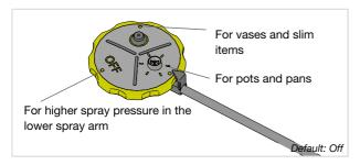
Leave the power zones open if you want an increased water flow where, for example, you have placed pots and pans or vases and slim items. Turn the dishwasher's power zones off if you want greater spray pressure in the lower spray arm.
