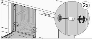
After fastening the machine, check that the front feet still touch the floor.
