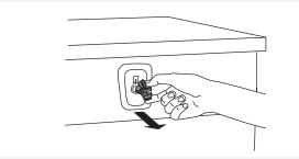
**2** To remove the plastic plugs holding the bolts, squeeze them and then pull them out.
