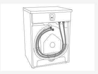
The water intake hose has to be fastened firmly enough for the hose to have a good seal.
