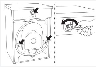
Release and remove the bolts as shown in the figures.
