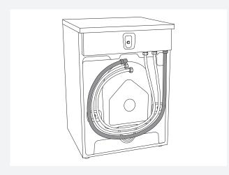
The machine is supplied with the outlet hose already attached. The hose should be extended over a suitable sink edge or drain pipe at a height of 24" to 36" (610 mm to 914 mm) above the bottom of the unit. (The lower height is preferable.) Make sure the hose is not kinked.
