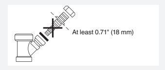
If the hose is extended, the internal diameter of the coupling must not be less than ½" (12.2 mm).
