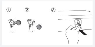
Remove the caps from the plastic plugs. Push the caps over the three holes in which the plastic plugs were inserted. Save the bolts and plastic plugs if you have to transport your washing machine in the future.
