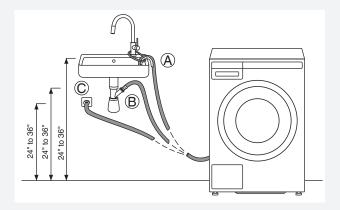
Drain hose can also be connected directly to the washbasin drain via a siphon. In this case, the hose, too, should be 24" to 36" (610 mm to 914 mm) above the floor. Internal hose diameter should be at least 0.71" (18 mm).
