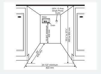
If the drain outlet is higher than 24"(610 mm), the connections will need to be recessed.
