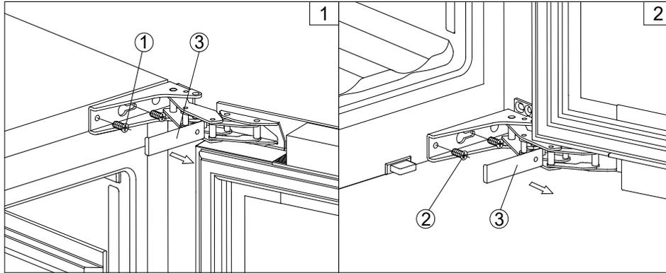
1. Remove the cover caps (3) and then remove the door by unscrewing the four screws (1) and (2). Be careful to hold the door firmly after removing the screws and place it on a padded surface to avoid the risk of damage.
