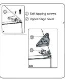
3. Remove screws ① and hinge ②. When the refrigerator with a display on the door, you need to pass connector ③ through the hole of the hinge ②. (Hold the upper door by hand when installing).
