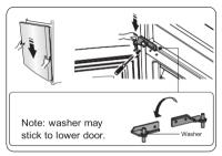
Move the upper door to an appropriate position, and then fix
