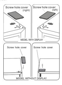
6. If the refrigerator with a display on the door, remove part ① from the top left side of the upper cover and take out part ②. Then remove part ③ and put part ④ into the top right side of the upper cover. Refer to the above operation, install part ③ and part ④ on the top left side of upper cover. Install part ① of the top right side of the upper cover. When the refrigerator is without a display on the door, skip this step.
