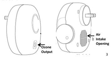
3. After removing loose debris using vacuum process. Lightly dip a cotton swab in isopropyl alcohol, insert the cotton swab into the ozone outlet opening. Gently rotate the swab while moving the swab in and out until all visible soil is removed. Use a dry swab and repeat above process to remove excess alcohol. Turn unit face down and allow the unit to dry 30 minutes.
