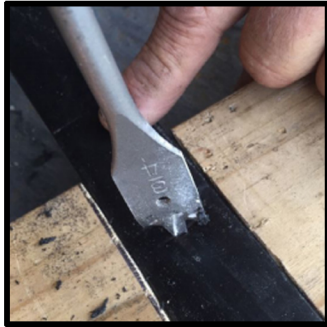
Use a 3/4" hole saw or 3/4" drill bit to cut the holes for the aluminum spacers
