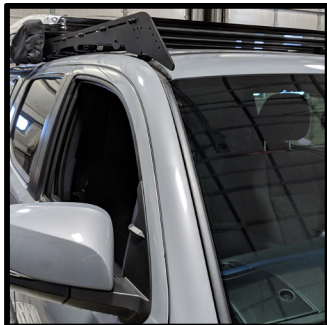
You can now place the roof rack on your vehicle and fully tighten down
