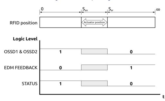
Figure 5 - OSSD / EDM / STATUS - logic levels
