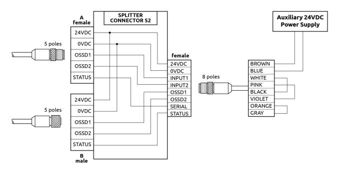
Figure 9 - Special connection for the auxiliary power supply
