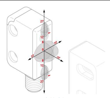
Figure 17 - Detection field of the sensor
