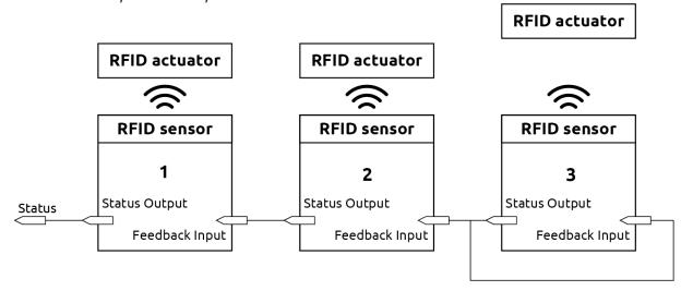
Figure 13 - Serial status modality encoding
