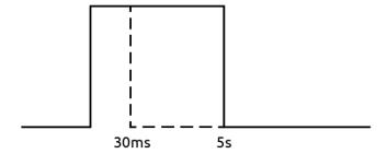
Figure 22 - Correct RESTART pulse
