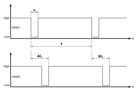
Figure 28 - Timing of OSSD test pulses
