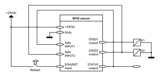
Figure 21 - Manual mode without EDM
