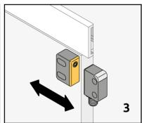
Figure 15 - Actuation direction
