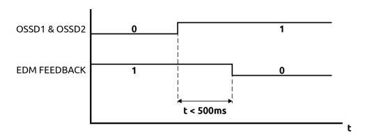
Figure 24 - Correct EDM timing
