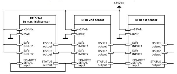
Figure 26 - First sensor in a serial connection
