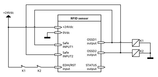
Figure 23 - Automatic mode with EDM
