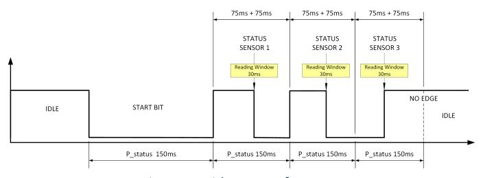
Figure 14 - Serial status waveform output
