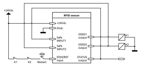
Figure 20 - Manual mode with EDM
