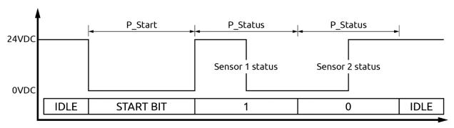
Figure 11 - STATUS serial asynchronous transmission
