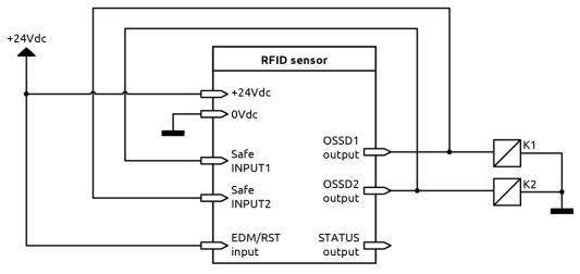
Figure 25 - Automatic mode - no EDM
