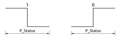
Figure 12 - Serial bit encoding
