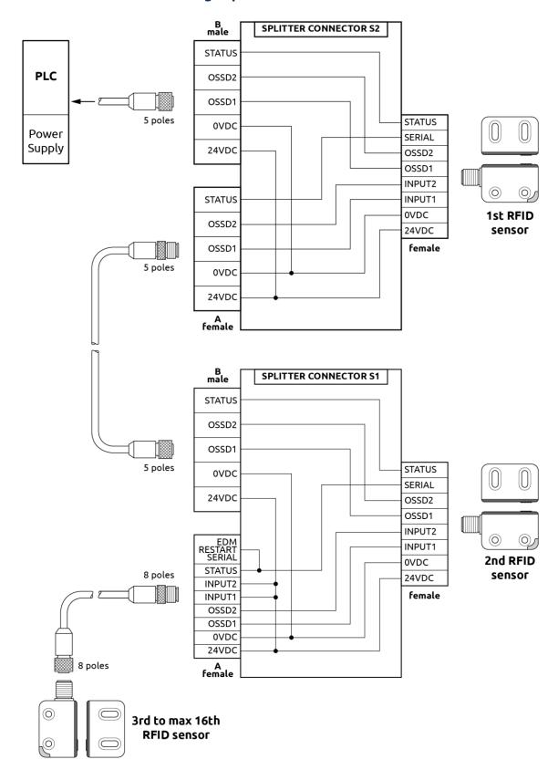
Figure 10 - Serial mode wiring (Automatic)
