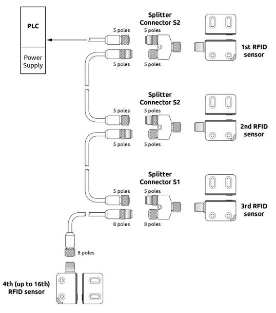
Figure 7 - Serial mode (Automatic)
