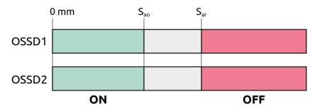
Figure 4 - OSSD outputs - logic levels
