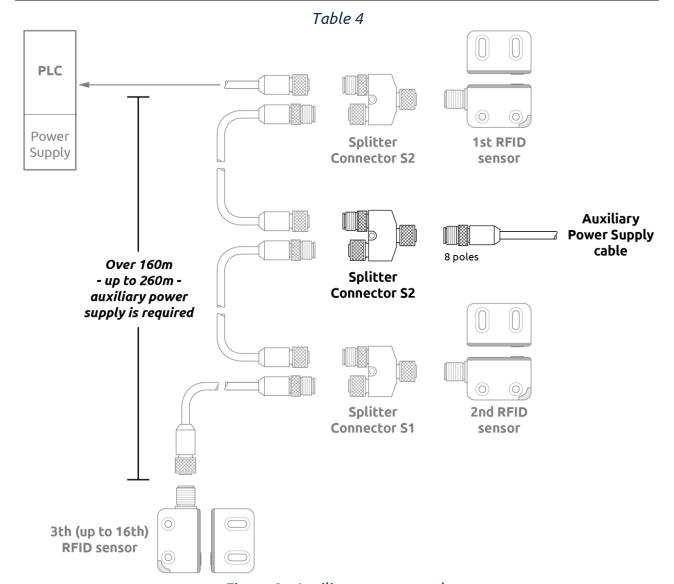
Figure 8 - Auxiliary power supply
