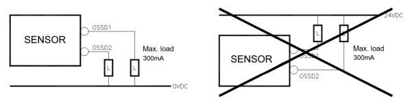
Figure 6 - Correct load connection on OSSDs
