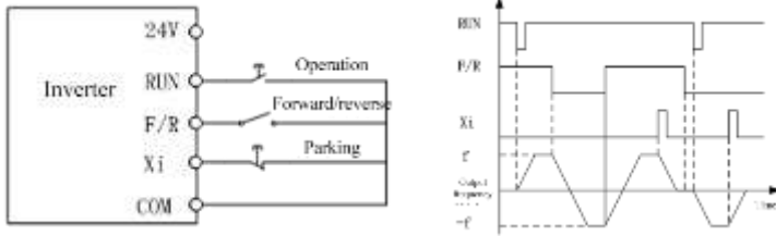
(c) Wiring diagram of three-line control (F00.03=3) (d) Forward/reverse running logic
