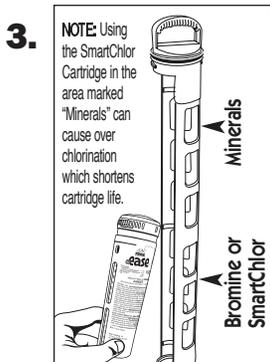
Snap the FROG @ease Mineral Cartridge into the area marked “Minerals” (top portion) and the FROG @ease SmartChlor Cartridge into the area marked “Bromine or SmartChlor” (bottom portion) making sure to line up the indentation at the top of the cartridges with the raised area on the holder.
