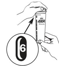
**Set the FROG @ease Mineral Cartridge** to #6 (hold the bottom and turn the top until 6 appears in the window). No further adjustments are necessary for the life of the cartridge.
