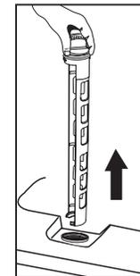
Remove holder by pushing down and turning counter clockwise 1/8th turn before pulling out.
