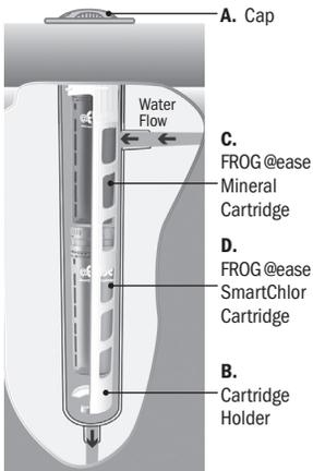
The In-Line System is made up of:
