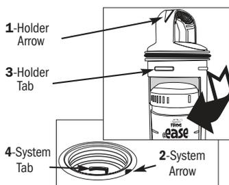
Slowly insert holder into system. Line up **holder arrow (1)** with **system arrow (2)**. Push down until **holder tabs (3)** go past **system tabs (4)** and turn holder to the right (clockwise) until it stops. To ensure a locked position, attempt to pull holder up. If it stays in place, the lock is secure.
