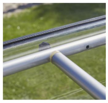
Fasten the rest of the frame to the hull using the washers, handknobs and metal retaining screws.
