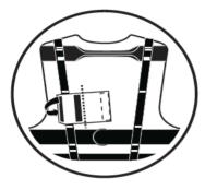
4. Place the folded tether in-line with the vertical strap. Bring the hook end around the tether and connect to the loop on back. Connect the carabiner to the D-ring on the rescue belt.
