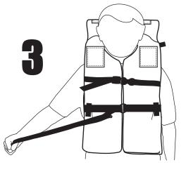
Pull free end of the top and bottom straps to adjust for a snug fit
